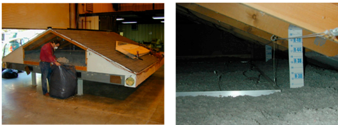
Figure 7. Large-scale climate simulator (LSCS) box test module ( left ); PCM-enhanced cellulose insulation ( right ).
